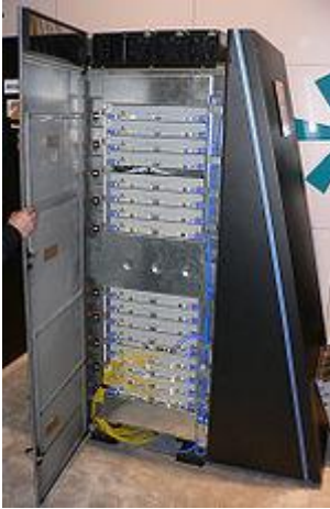
Figure1.10. A Blue Gene / L cabinet with stacked blades, each with multiple processors.
